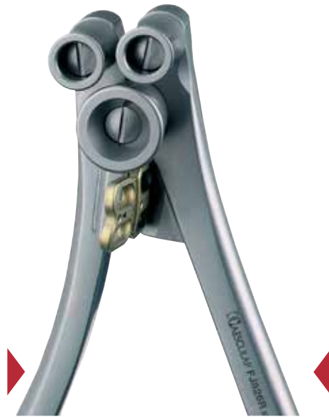
Fig. 15: Plate curvature can be reduced by using the bender in this manner.
